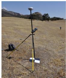
Above: Trimble R8 survey-grade GNSS rover set up on a ground control point along the San Andreas fault near Dry Lake Valley, California. We use the R8 in VRS, RTK, and fast-static mode, depending on the situation, to obtain control point locations with 1 to 2 cm 2-sigma accuracy.
