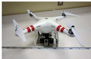
Above: DJI Phantom II quadcopter, GoPro Hero 3 Black Edition camera, and Zennuse H3-3D gimbal used for acquisition of aerial photographs. The UAV is equipped with a WiFi system that relays video from the GoPro to a ground-based monitor in real time to aid navigation and positioning of the UAV during flights.
